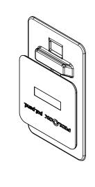
total possible material thickness between male and female part: 3mm depends on way of assembly,
