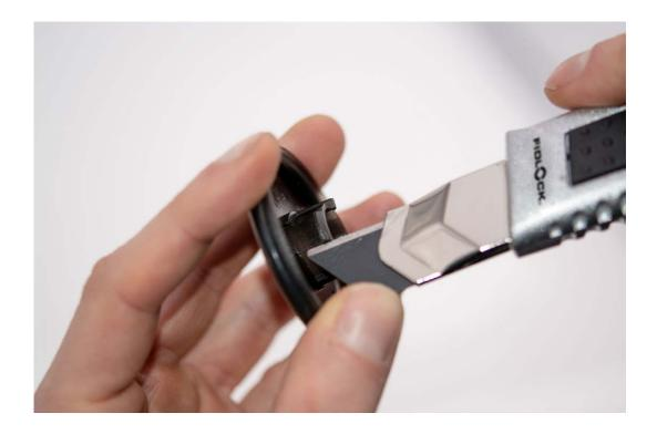
The MINITURN handle features a single-use catch mechanism and cannot be removed once it has been successfully fitted! For prototypes and testing, the handle can be made removable by cutting off two catch hooks, as shown in the image below.
